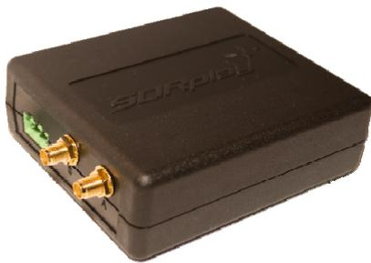
Bild 15: SDRplay RSP2, SDR-Receiver
