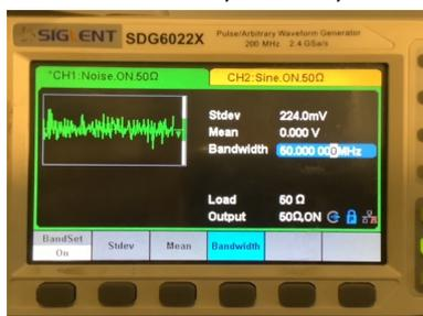
True RMS Voltmeter, 224mVeff, 1mW an 50 Ohm
