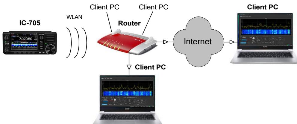
Figure 2: IC-705 does not need a server PC because WLAN and server are already integrated
