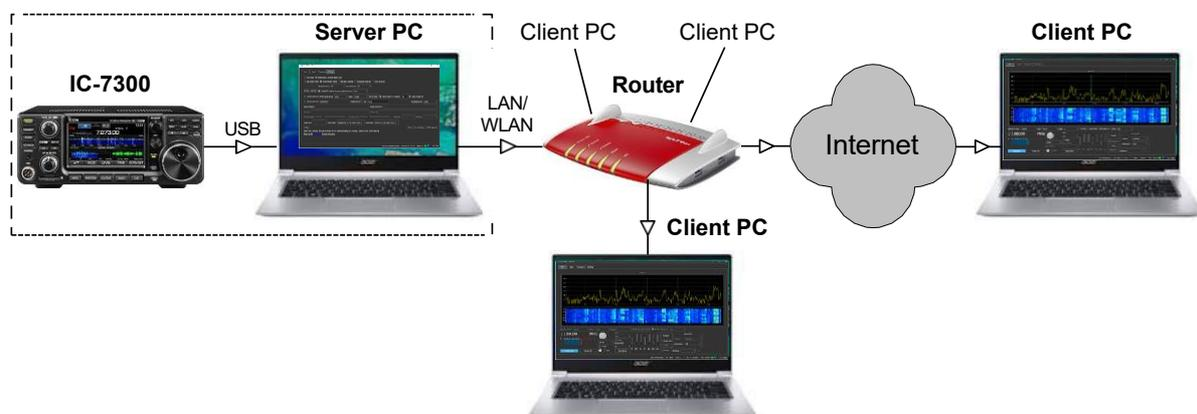
Figure 1: IC-7300 requires a server PC for remote control
