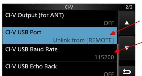
Figure 3: Settings on the IC7300 USB
