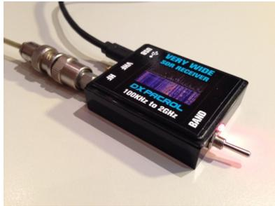
SDR Receiver DX Patrol, 100kHz-2GHz
