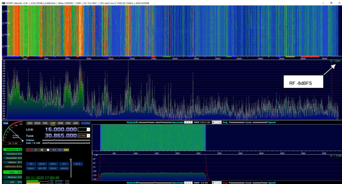
Figure 8: HF reception from 0-32MHz with high transmission speed
