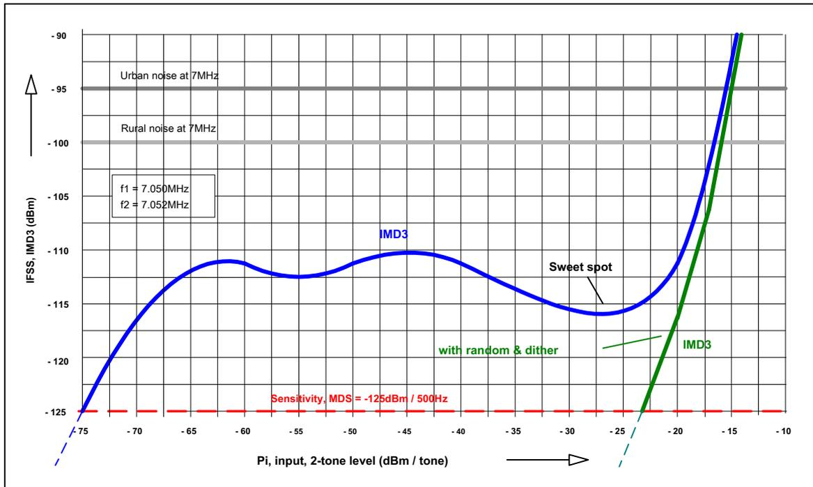
Figure 9: 2-tone IMD3 test, f1 = 7,050MHz, f2 = 7,052MHz, delta f = 2kHz
