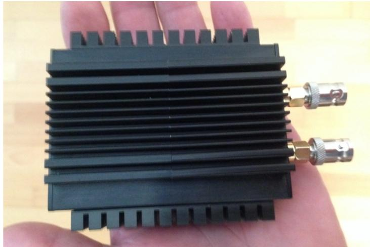
Originally the RX666 (BBRF103) was designed by Oscar Steila (Turin), under the name DRAGONFLY (<http://www.teila.com/blog/>). It is a direct sampling 16bit SDR that transmits signals from 1kHz to 32MHz in real time with 64Mbps sampling rate and can be used up to 1.8GHz via the built-in R820 chip.
