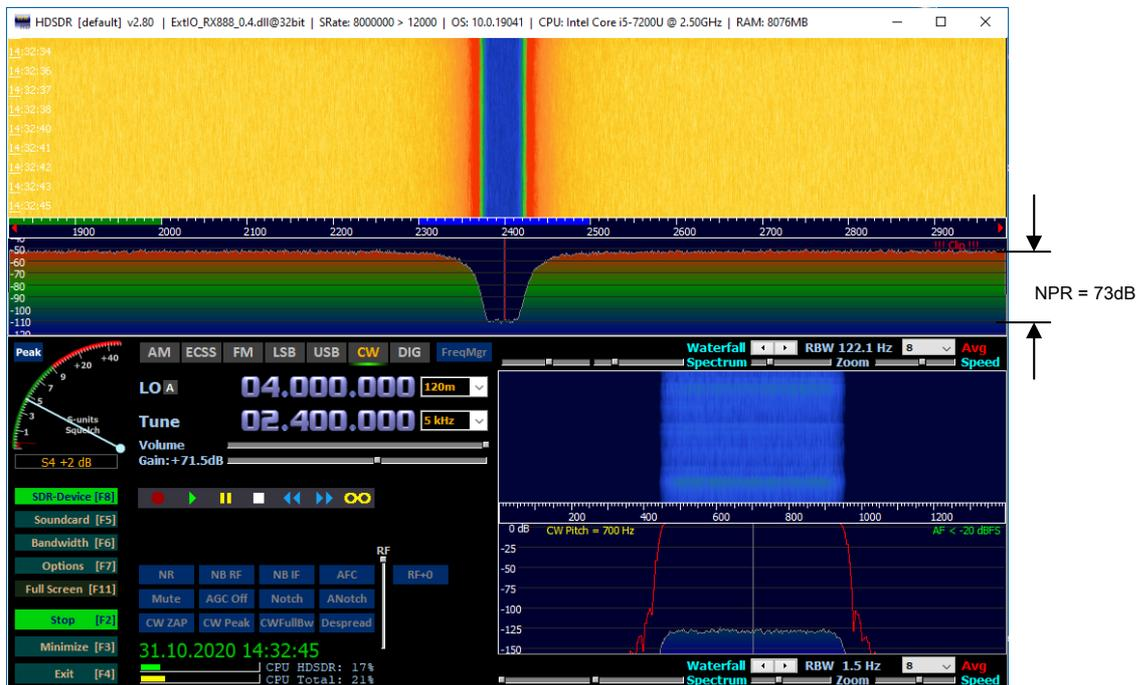
Figure 11: Maximum NPR with a noise level of P<sub>TOT</sub> = -12dBm
